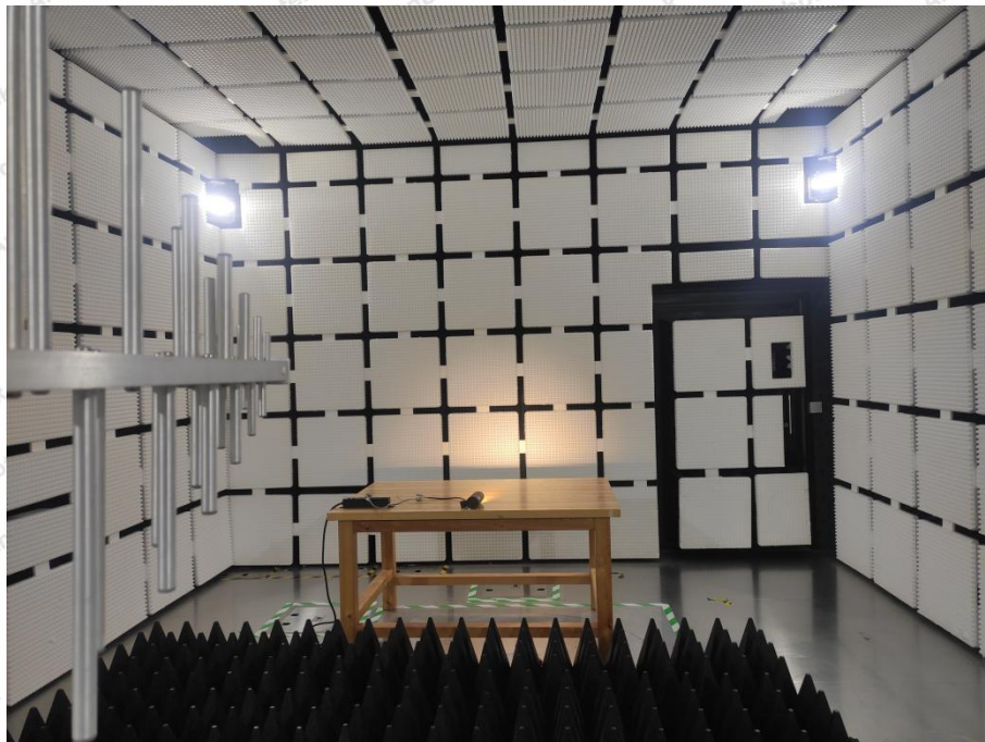
Photo of RF Field Strength Immunity Test
